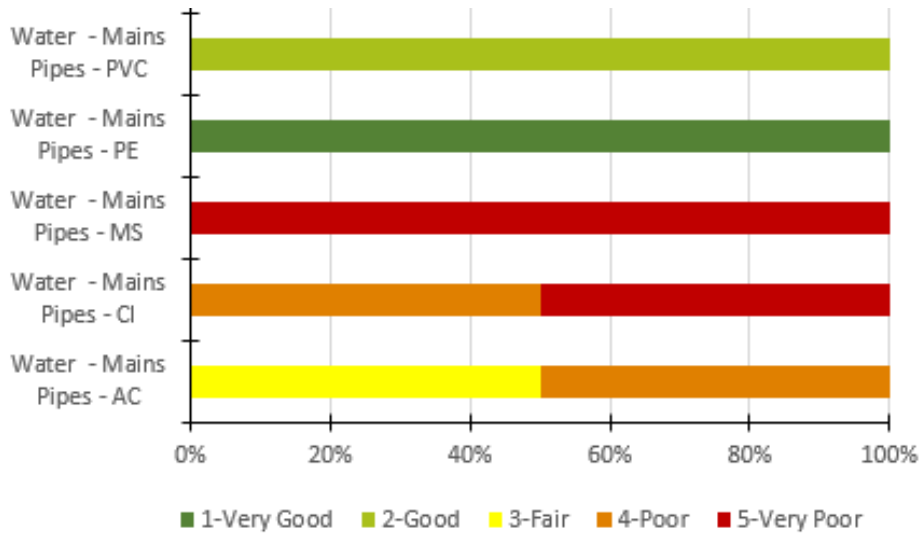
Figure 4: Condition Profile – Water Mains
