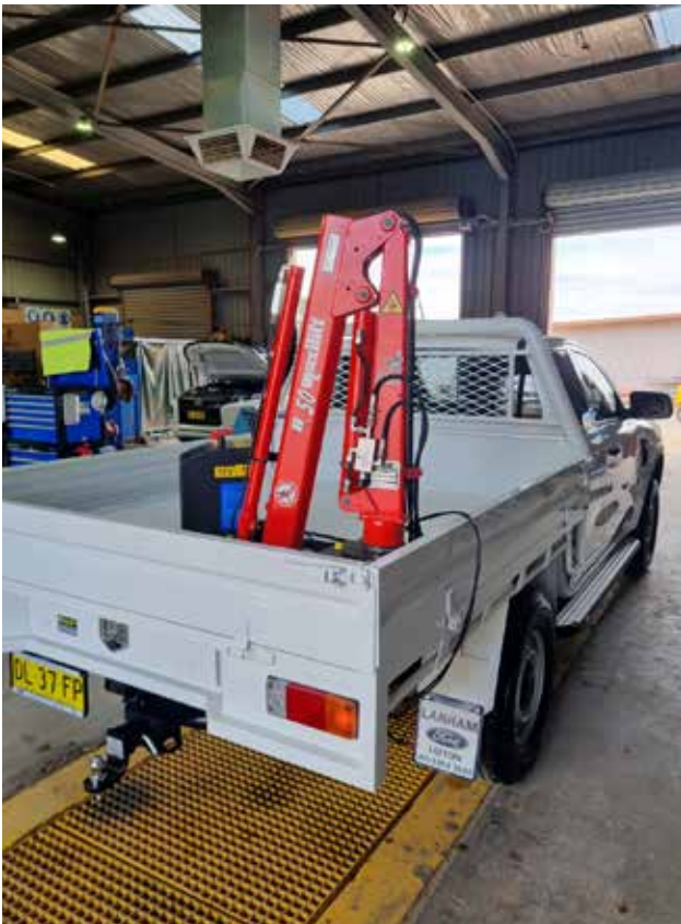
Lifting units for the utes to alleviate manual labour
