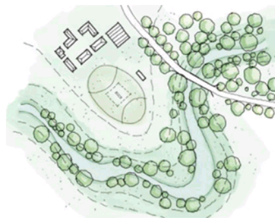
Diagram 2 - Land use and built form avoids land that is environmentally constrained. Image Source: Draft Urban Design Guideline - NSW DPE
